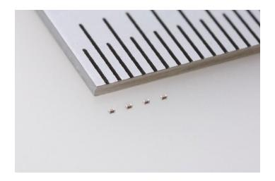
TOKYO, March 8, 2017—TAIYO YUDEN CO., LTD. has begun mass production of the world's smallest 0201 size (0.25 x 0.125 x 0.125 mm) high frequency multilayer ceramic capacitors.
