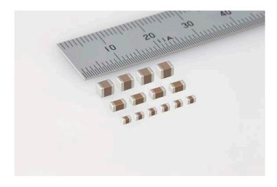
TOKYO, January 29, 2014 — TAIYO YUDEN CO., LTD. today announced the commercialization of resin external electrode multilayer ceramic capacitors "HMJ212BB7104KGHT" ( $2.0 \times 1.25 \times 1.25 \text{mm}$ ), "HMJ316BB7105KLHT" ( $3.2 \times 1.6 \times 1.6 \text{mm}$ ), and "HMJ325AB7225KMHT" ( $3.2 \times 2.5 \times 2.5 \text{mm}$ ) that use a conductive resin for the external electrodes of the multilayer ceramic capacitor.
