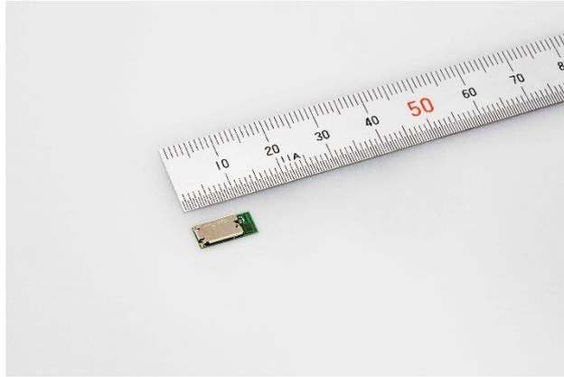
TOKYO, October 1, 2019—TAIYO YUDEN CO., LTD. announced today the launch of the new *Bluetooth*<sup>®</sup>\*1 5 compatible wireless communications module, EYSKJNZWB (5.1×11.3×1.3 mm). This product is most suitable for IoT-related devices that are required to be small and thin, such as wearable terminals, healthcare devices, and physical distribution terminals.
