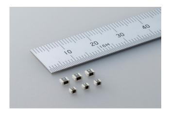
TOKYO, June 27, 2022—TAIYO YUDEN CO. LTD. has announced today the launch of the wire-wound metal power inductor MCOIL<sup>TM</sup> LCEN series. Qualified for AEC-Q200 (reliability qualification test standard for automotive passive components), the series consists of 13 items in two sizes, including the LCENA2016MKTR24M0NK (2.0x1.6x1.2 mm, height is the maximum value).
