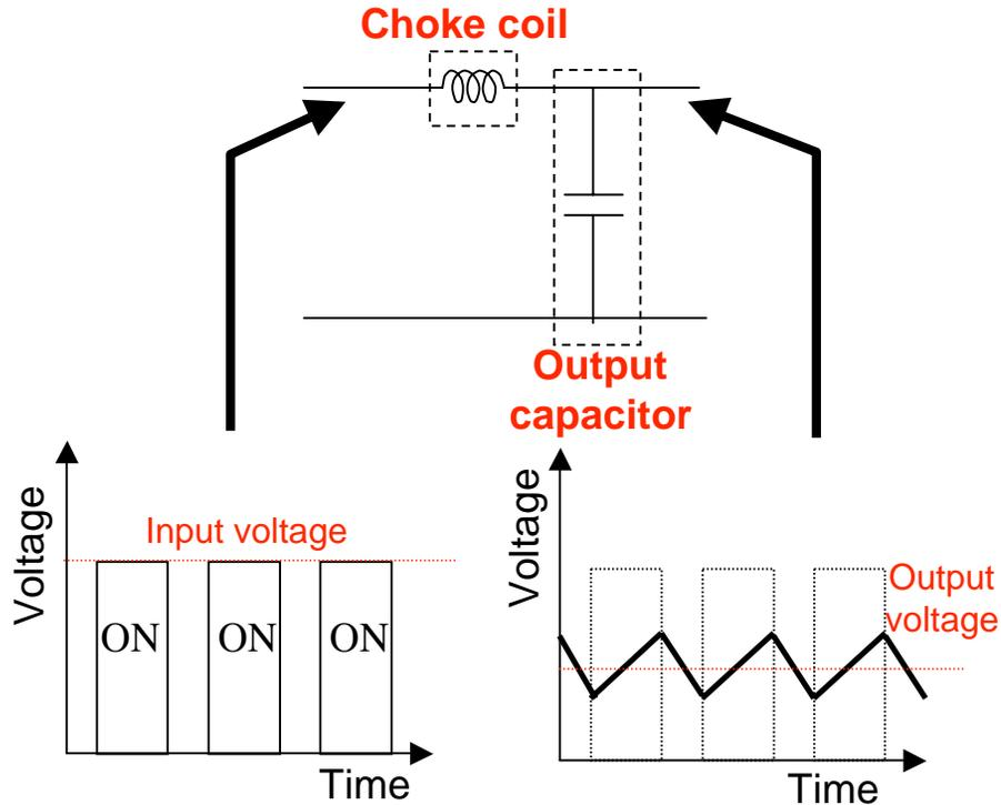
Input voltage is controlled by an on-off switching.
