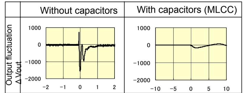
Output voltage is stabilized as output capacitor is connected.
