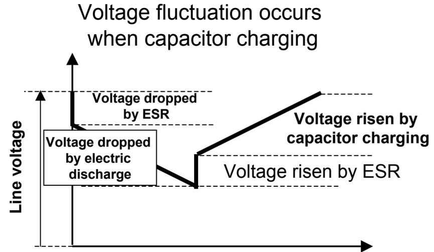
Keeping the minimum required operational voltage for IC  $\Rightarrow$  Maintaining stable operation
