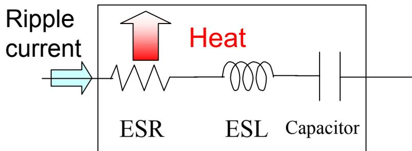
Electrical energy is converted to **heat** when **ripple current** (AC) goes through capacitor. (DC does not go through it)
