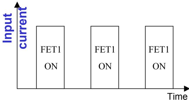
Large amount of alternating current (ripple current) flows.
