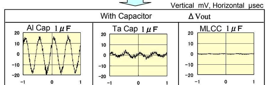
Output fluctuation becomes smaller as IC input voltage stays constant.
