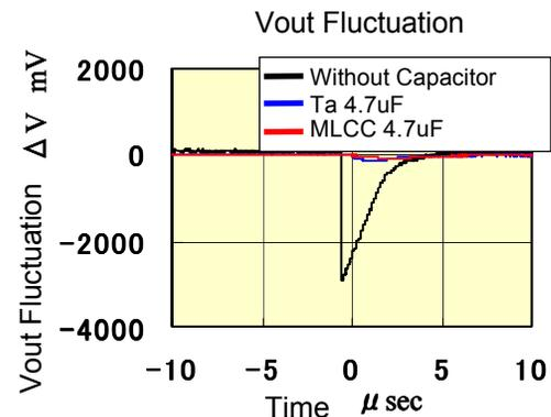
Waveform observation:  $I_{out}$ ,  $V_{out}$
