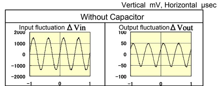
Input fluctuation of 1Vrms → Output fluctuation of 35Vrms
