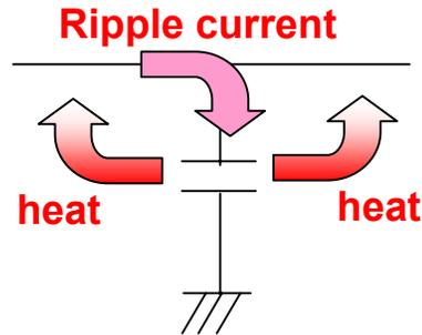
Ripple current flows into input capacitor.
