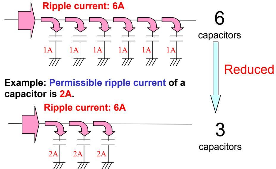
Example: Permissible ripple current of a capacitor is 2A.
