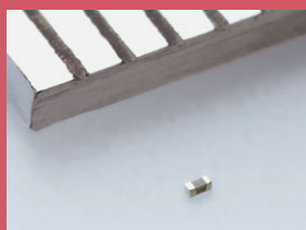
008004 size (0.25 mm × 0.125 mm) ultra-small multilayer ceramic capacitors
