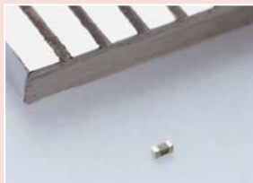
008004 size (0.25 mm × 0.125 mm) ultra-small multilayer ceramic capacitors
