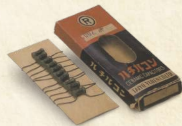
Rutilcon, barium titanate tubular ceramic capacitors
