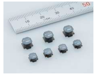
Ferrite-base wire-wound power inductors
