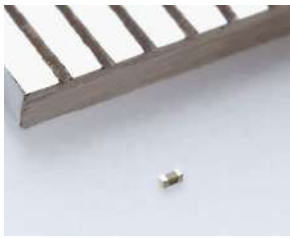
0201 size (0.25mm×0.125mm) ultra-small multilayer ceramic capacitors
