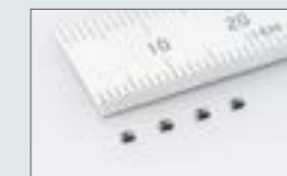
Multilayer metal power inductor "MCOIL™ MC Series" (1.6mm×0.8mm×1.0mm, 0.47µH)
