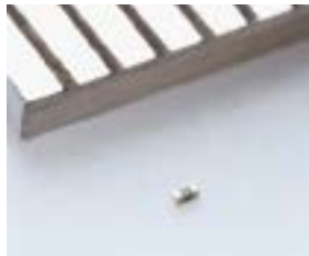
0201 size (0.25mm×0.125mm) ultra-small multilayer ceramic capacitors
