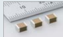
4532 size (4.5mmx3.2mm) with 1,000µF capacitance
