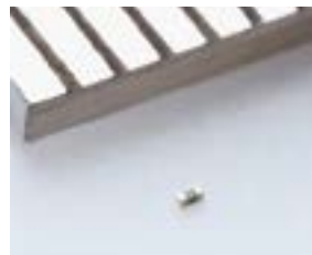
0201 size (0.25mmx0.125mm) ultra-small multilayer ceramic capacitors
