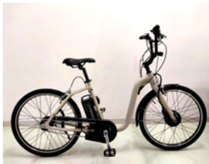
Regenerative electric assist system "FEREMO™" for electric assist bicycles
