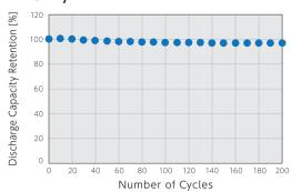
Charging: 1.0 mA / 3.65 V (CCCV) – terminated after 10 hours Discharging: 0.5 mA (CC) – terminated at 2.0 V Environment:  $25^{\circ}$  C
