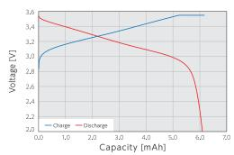
Charging: 1.0 mA / 3.55 V (CCCV) – terminated after 10 hours Discharging: 0.5 mA (CC) – terminated at 2.0 V Environment: 25° C
