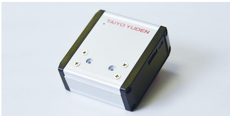
▲QCM-type prototype smell sensor under development
