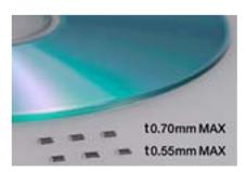
Taiyo Yuden announces a new multilayer choke coil, the CKP3216L (EIA 1206,3.2 x 1.6 x 0.55mm) and the CKP3216M (3.2 x 1.6 x 0.70mm), used in DC-DC converters for mobile equipment (in both cases, the height represents a maximum value). CKP3216L, in particular, marks the advent of the thinnest multilayer choke coil in the industry for DC-DC converters.
