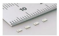
Taiyo Yuden announces the 0805 size  $(2.0 \times 1.25 \times 0.5 \text{mm})$  maximum thickness) low pass filter, thinnest in the industry, made for use in mobile equipment tuners for terrestrial digital TV broadcasts.
