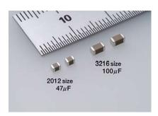
Taiyo Yuden will commence mass production in July 2005 of a  $100\mu F$  compact, high-capacitance multilayer ceramic capacitor in the EIA1206 size (3.2 x 1.6 x 1.6mm) and a  $47\mu F$  capacitor in the EIA0805 size (2.0 x 1.25 x 1.25mm). The move to mass production is an industry-first for both products.
