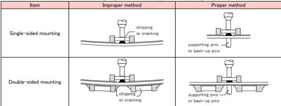
2. As the alignment pin wears out, adjustment of the nozzle height can cause chipping or cracking of the inductors because of mechanical impact on the inductors. To avoid this, the monitoring of the width between the alignment pin in the stopped position, and maintenance, inspection and replacement of the pin should be conducted periodically.
