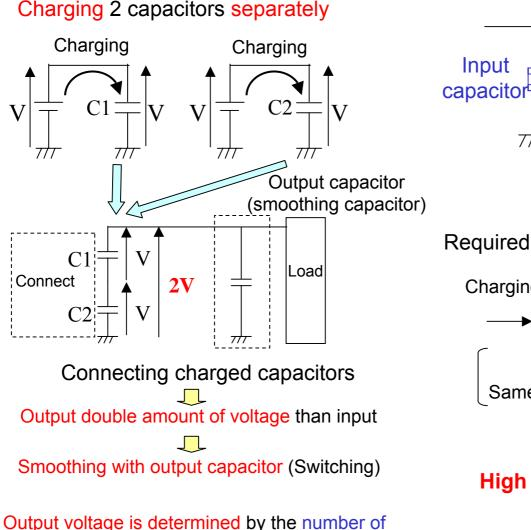
capacitors connected. (integral multiple)
