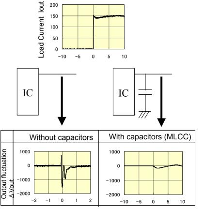
Supply current to control voltage fluctuation for rapid load change
