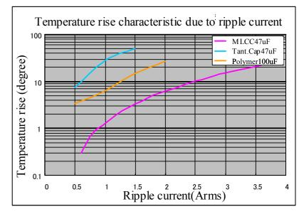
Given the same amount of calorific power, ripple current goes through MLCC the most because of its low ESR.
