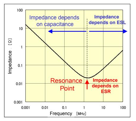
At resonance point, no impedance for Capacitor & ESL (Impedance for ESR only)
