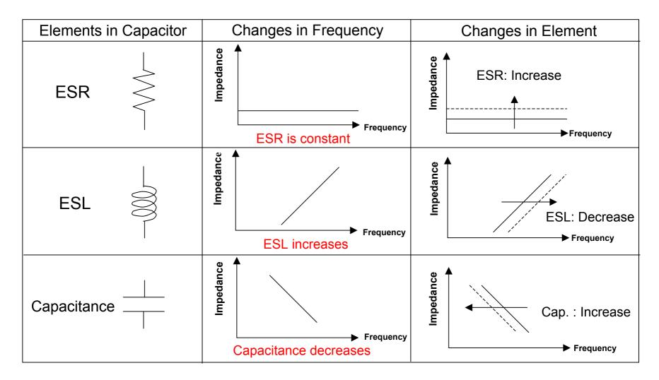
What happens to the impedance level when connected in series?
