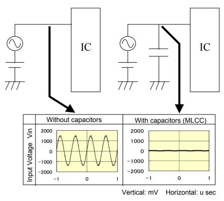
Same as the function of Bypass Capacitor Input voltage is stabilized as input capacitor is connected.
