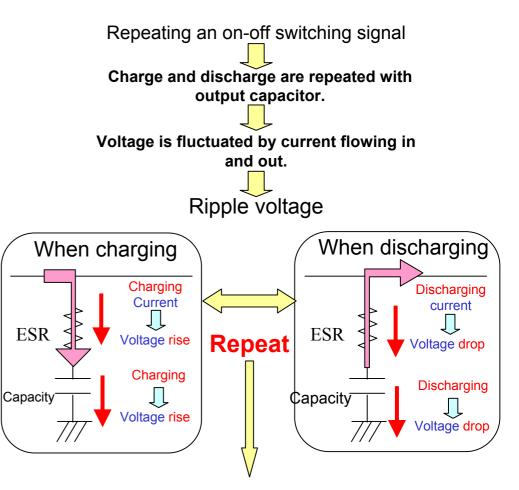
High capacitance and low ESR reduce ripple voltage.
