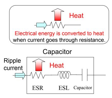
Electrical energy is converted to heat when ripple current (AC) goes through capacitor. (DC does not go through it)
