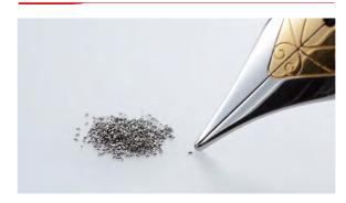
As a main product of TAIYO YUDEN, we are conducting research on a daily basis to further miniaturize while increasing the functionality of multilayer ceramic capacitors (MLCCs). There is a growing need for MLCCs to evolve in concert with the increasing miniaturization, functionality and power-saving qualities of electronic devices.
